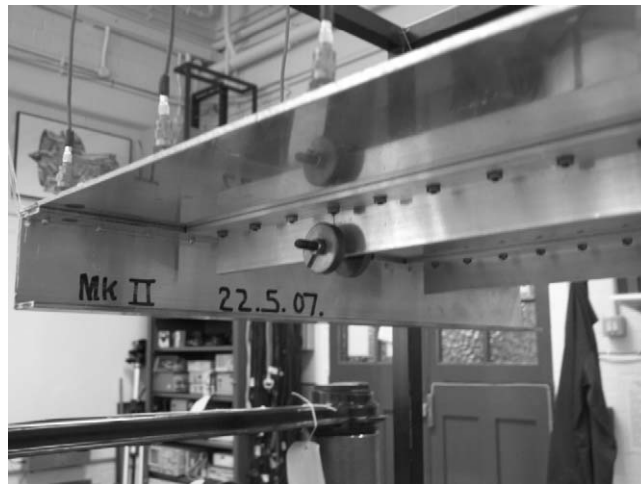
Fig. 15. Photograph of the 'aircraft wingbox' with mass added on one of its stringers.
